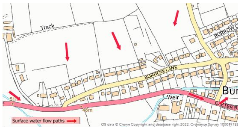
Figure 4.4 OS map marked to show the flow paths experienced in Burrow on 9 May 2023
