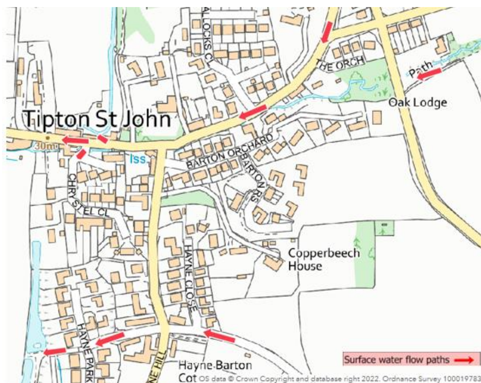
Figure 4.9 OS Map showing flow paths, marked by arrows, of surface water and Coombe Stream through Tipton St John during event
